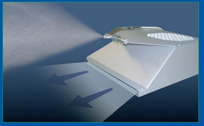
Eco-Mist systems feature humidifier units that combine high quality, stainless steel, non-drip nozzles, with low noise fans. A mist vortex is created where the airflow meets the mist, which evaporates guickly and completely.
